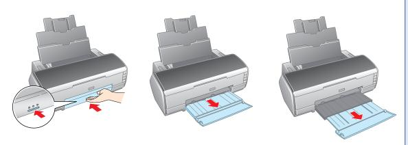
Fan a few sheets of paper and load them against the right side of the sheet feeder. Slide the left edge guide against the paper.
